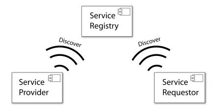
Figure 2.2. Discovery in Service-Oriented Architecture
