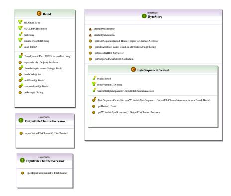
Figure 5.5. Object-oriented interface to byte store
