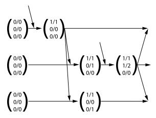
Figure 4.32. Dual-clock time vectors with local and global counter
