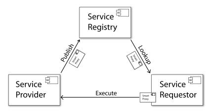
Figure 2.3. Execution in Service-Oriented Architecture
